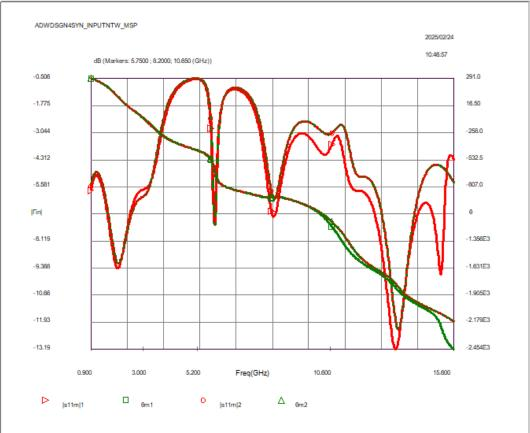
The input reflection coefficients of the load and input networks of the amplifier with implicit junctions are compared here with the reflection coefficients of these networks with S-parameter based junctions. The efficiency of the amplifier (ADW simulation) is degraded by 1% when the junctions in the load network is upgraded and by a further 1.5% when the input network is upgraded.
