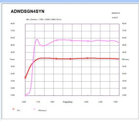
The performance of the ADW circuit in the previous slide as simulated in Microwave Office<sup>TM</sup>. The electrical circuit (ADW schematic) was simulated here to avoid distortions associated with differences in the microstrip models. These distortions can be reduced by using S-parameter based junctions in the ADW or by optimising the ADW microstrip networks in Microwave Office<sup>TM</sup> to fit the S-parameters of the ADW matching networks.
