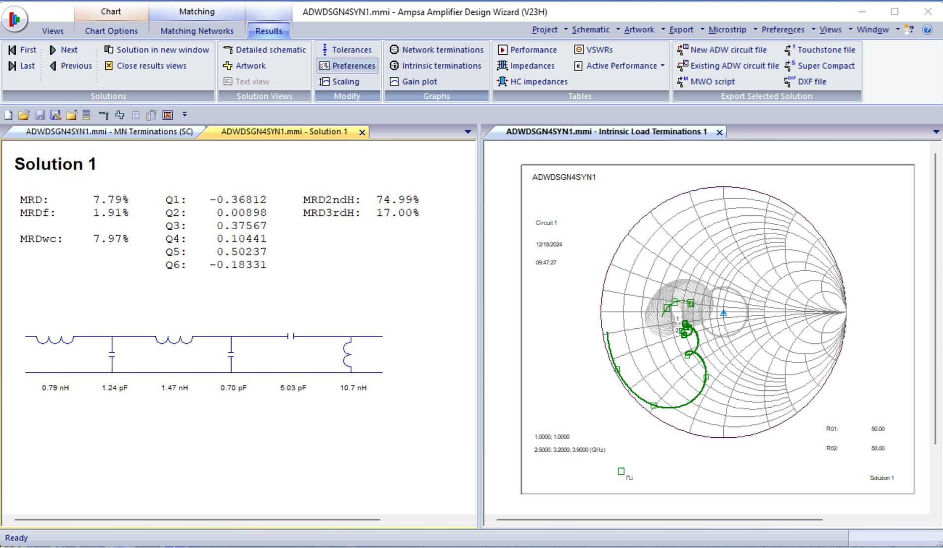
The effect of reducing the second harmonic transition band to 0.3 GHz is shown here.
