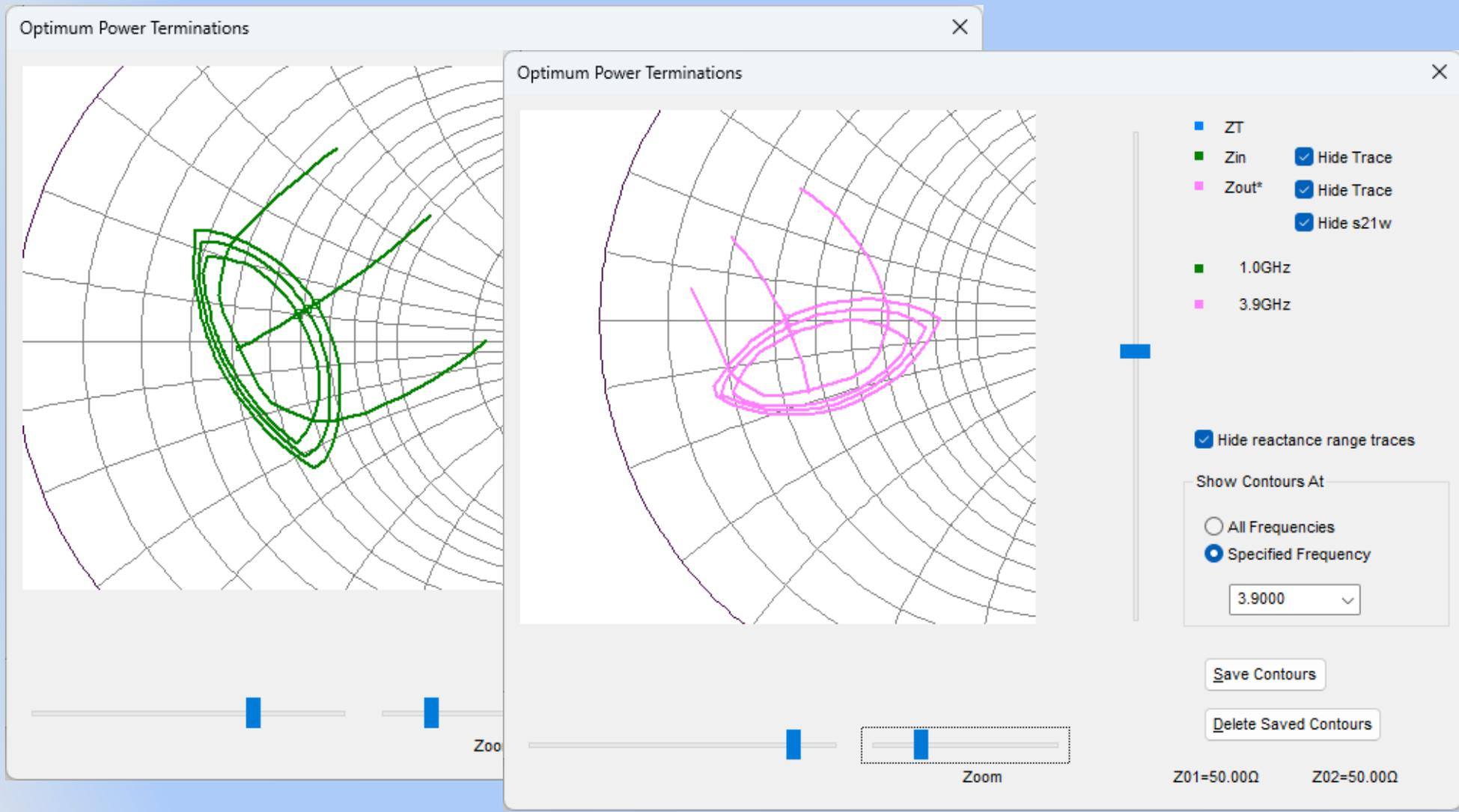
The constant power contours and the efficiency lines at 1.0 GHz and 3.9 GHz are displayed here.
