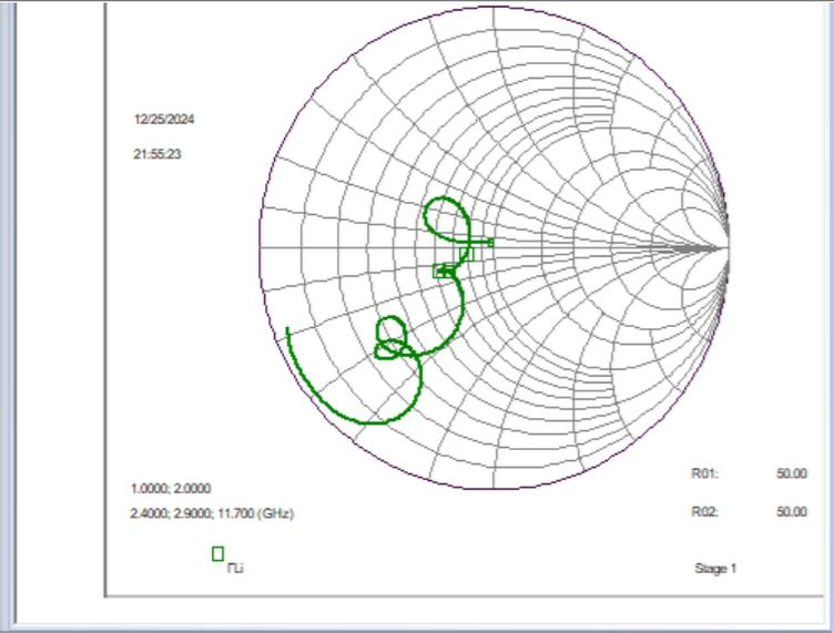
Use the Set Results Views command to set the views to be opened when an element value is tuned. The views can be arranged as required after using the Analyse command. The Summary Table command is used to tune the selected element value.
