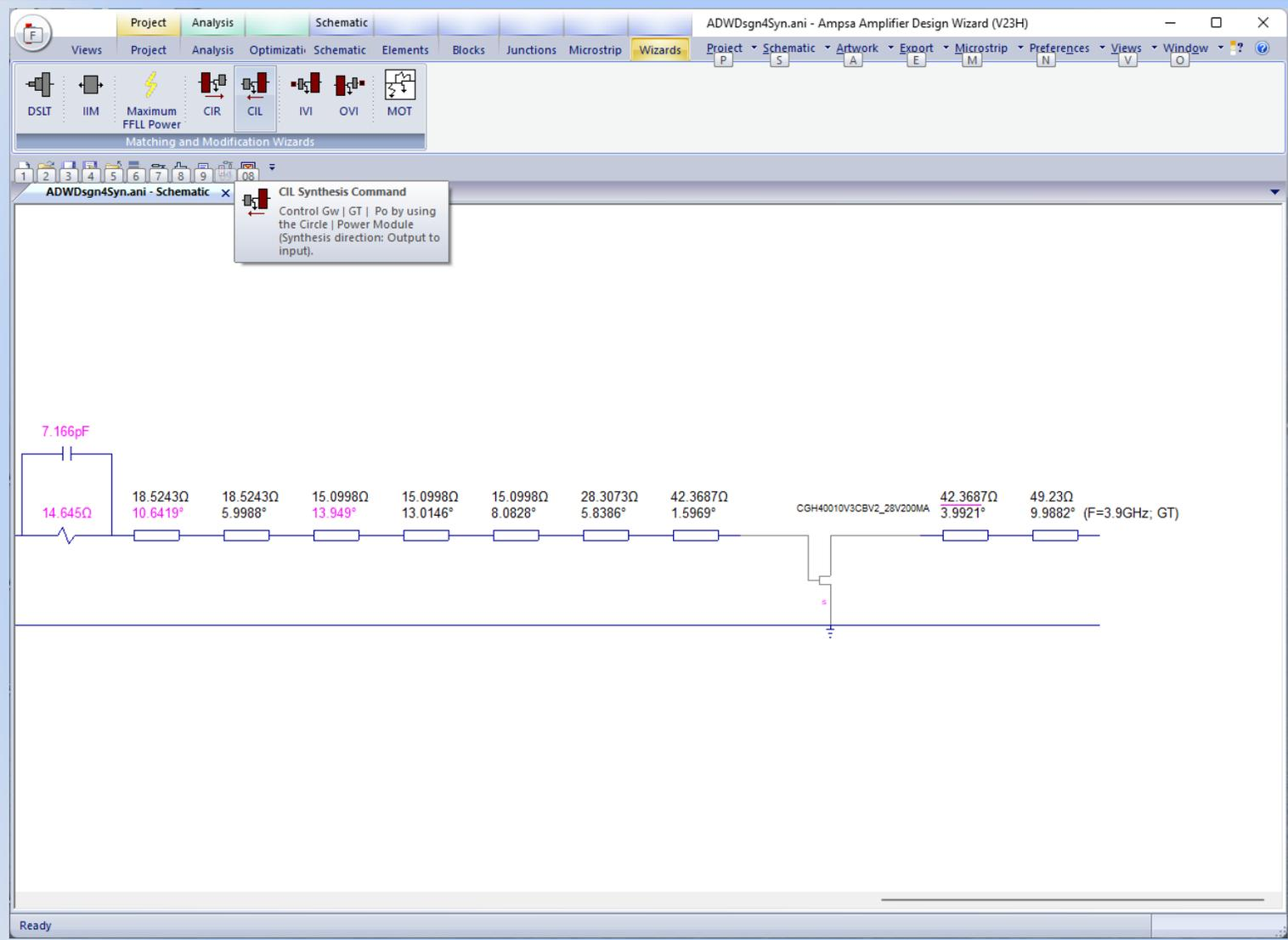
The ADW synthesis wizards must be launched with a schematic view active. The insertion point for the matching network required must be selected before launching the wizard.
