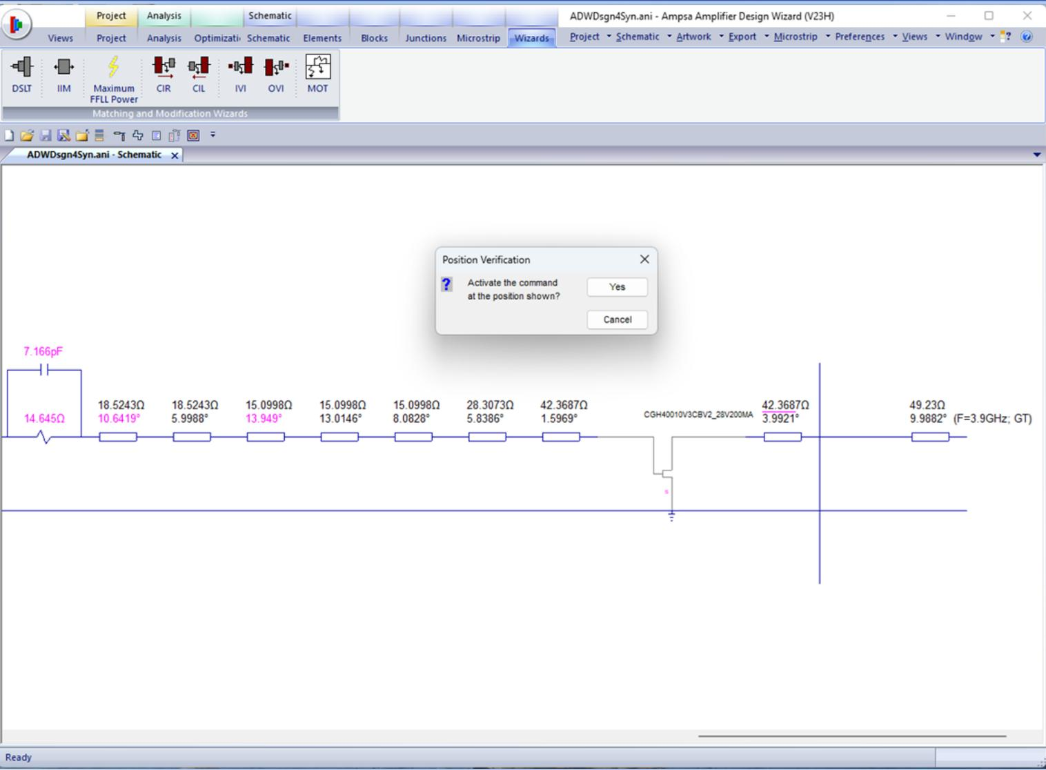
The CIL wizard was launched by selecting the Schematic | Wizards | CIL ribbon command. The schematic will be split as shown by the command.
