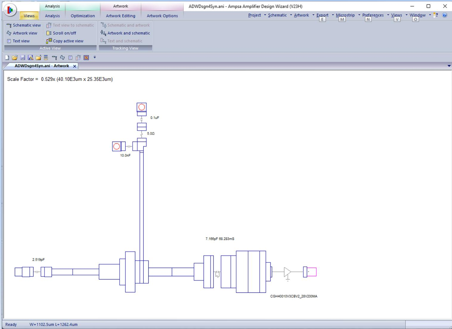
The circuit shown will be used as a starting point for the design. The input matching network is from a previous design, but the design flow is still valid without an input matching network in place. (Stabilizing the transistor, at least inside the passband is, however, advisable.) The input network can be optimised when the load network is in place.
