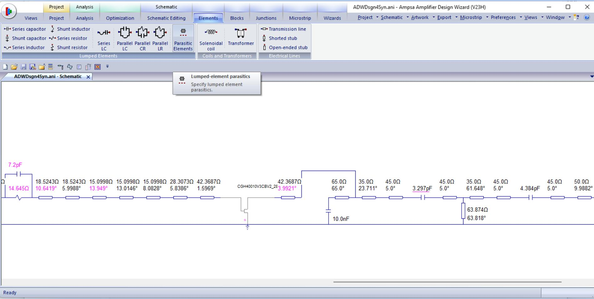
The lumped-element parasitics were ignored when this matching network was synthesized. Parasitic elements can be added to a capacitor by using the command shown after selecting the capacitor. The capacitor value can then be tuned to compensate for the inductance added.
