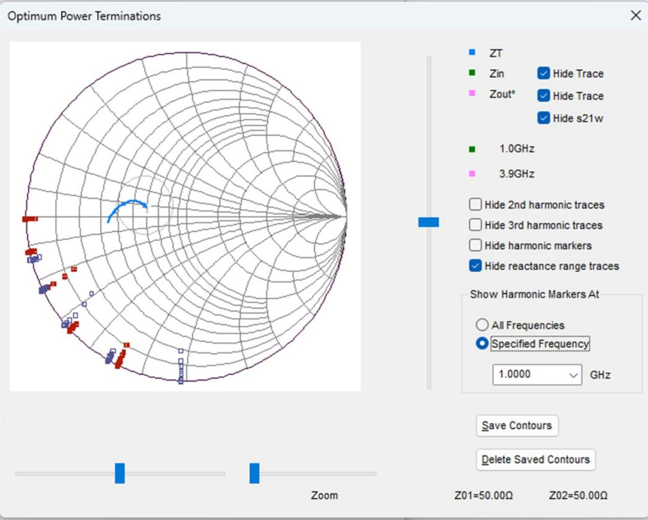
The targets can be displayed for all the passband frequencies or for a specific passband frequency. The associated intrinsic impedances will be near shorts for terminations at the centre of the range of external reflection coefficients shown for each harmonic.
