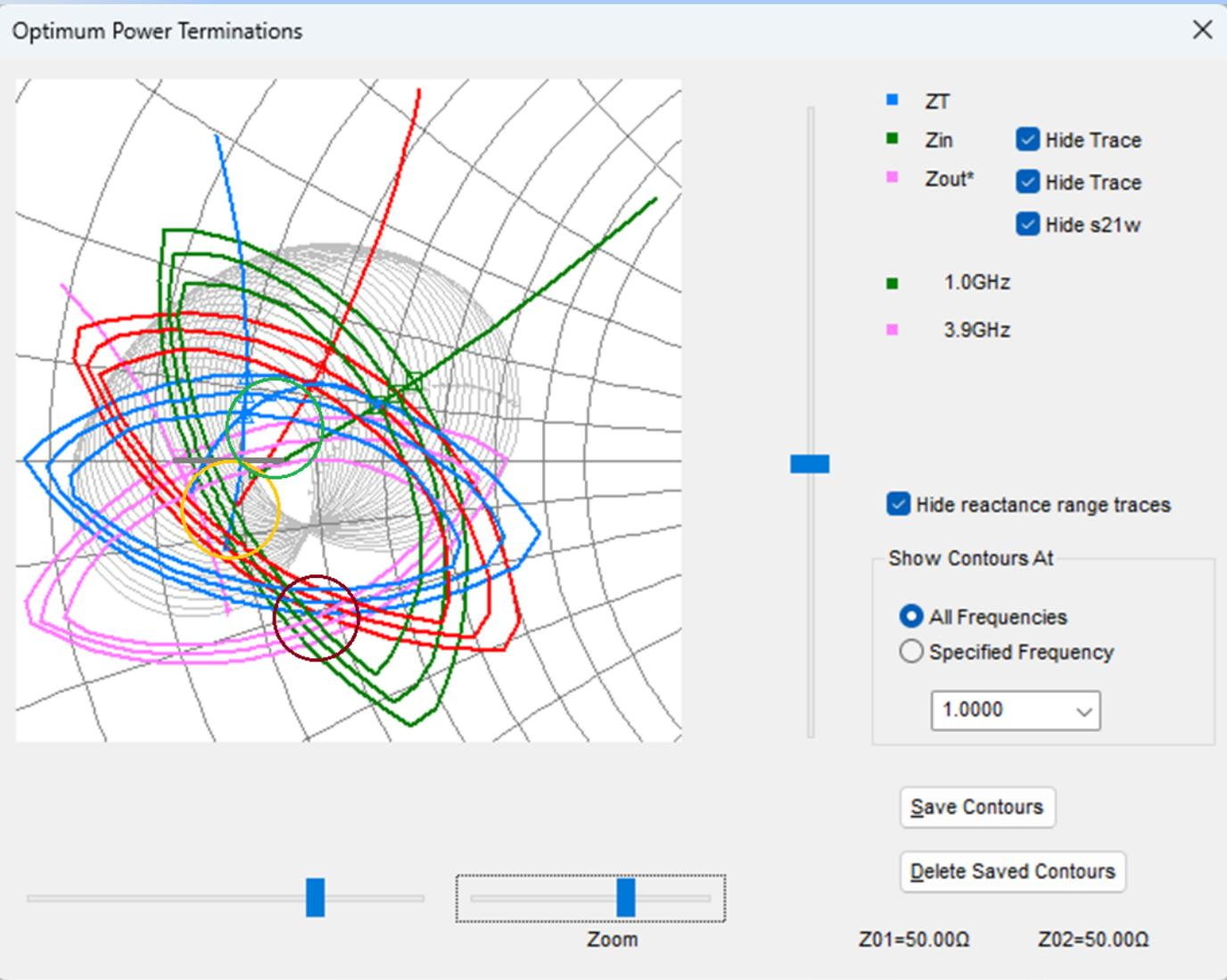
The Display Graph command provided on the wizard page was used to display the circles to be targeted in the Impedance-matching module. The constant power contours and the maximum efficiency lines are also shown.
